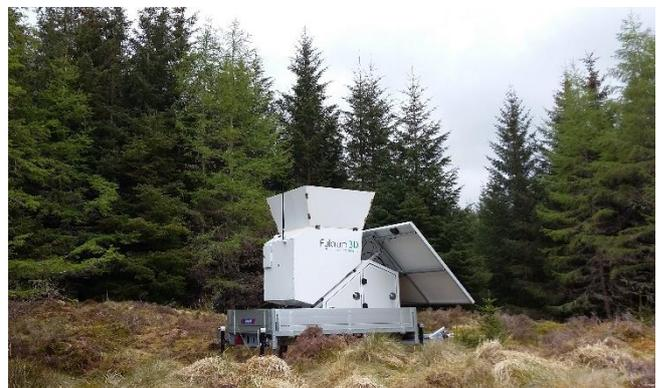
*Figure 12: Heavily forested monitoring location in Scotland, UK, complete with acoustic protection baffles*
