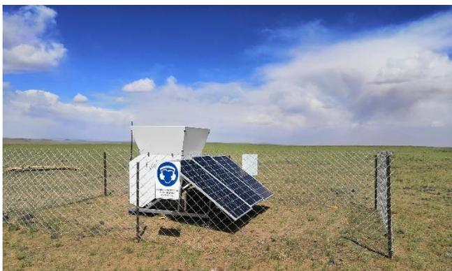
*Figure 11: Fulcrum3D Sodar operating in harsh environments in China*
