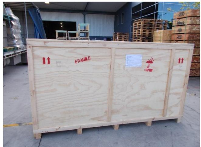
*Figure 4: International grade ISPM 15 stamped plywood casing*
