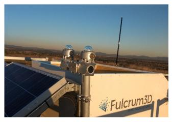
Figure 15: Solar monitoring kit - two Kipp & Zonen pyranometers
