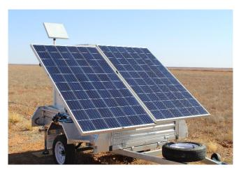
Figure 16: Satellite modem and antenna fitted for extremely remote monitoring in QLD
