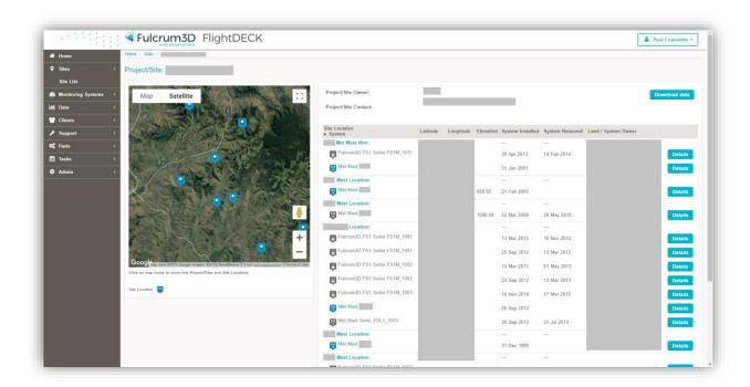
Figure 9: FlightDECK - Fulcrum3D Sodar and Met Mast Monitoring across a project
