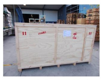
Figure 4: International grade ISPM 15 stamped plywood casing
